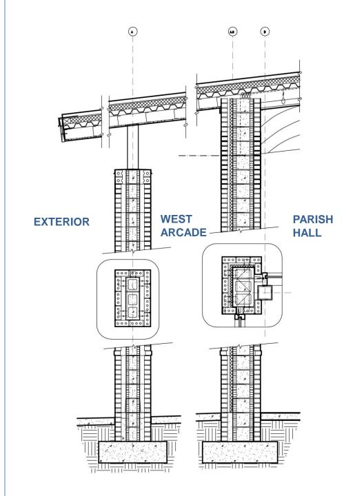
BRICK VENEER PROVIDED THE FORMWORK FOR THE POURED-IN-PLACE CONCRETE LINTELS OVER THE ARCADE AND GLASS OPENINGS
